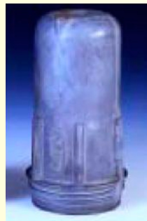
No corrosion with treatment
