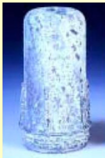
Rapid corrosion of untreated aluminium
